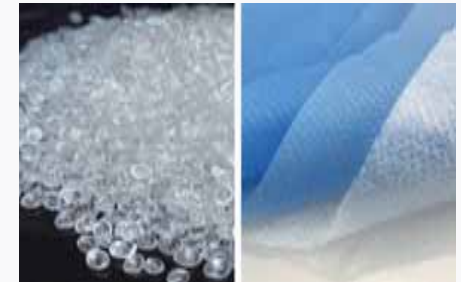
PLA Particles and Nonwovens Made of PLA
